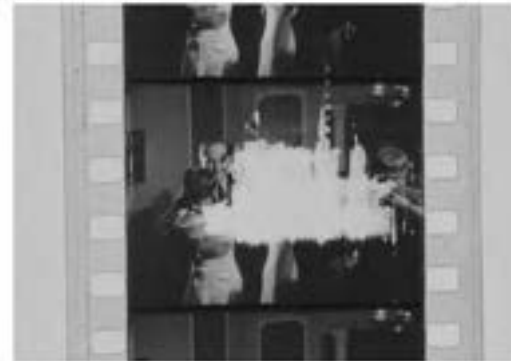
Emulsion detachment caused by film dragging and traction with projector
